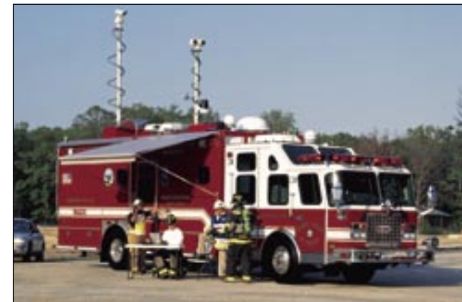
E-ONE built this well-equipped command vehicle for the Dumfries-Triangle Volunteer Fire Department, Va. It has communications gear, two extendible camera masts, a weather station and a command area.
