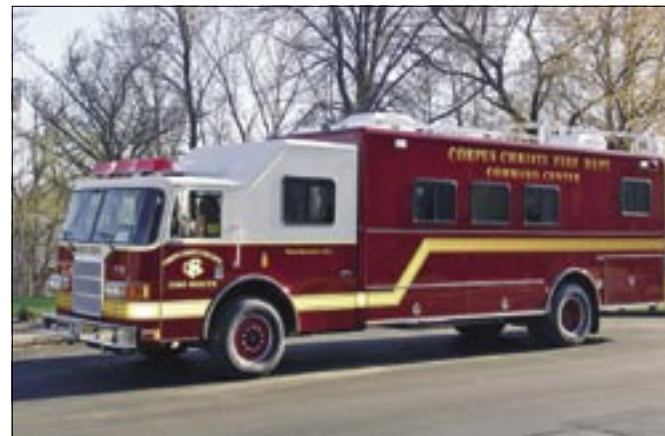
The Corpus Christi (Texas) Fire Department purchased this command center built on a Pierce Enforcer chassis. It has a five-person work area, conference room, surveillance camera, generator, toilet and observation deck.
