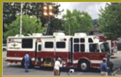
The San Ramon Valley Fire Protection District's new SVI communications support unit is equipped with five computer workstations. The stations are interconnected via a local-area network and have Internet access via satellite and the fire district's 802.11 WiFi system.
