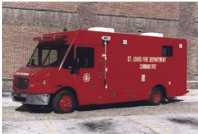
St. Louis, Mo., operates a mobile command post built on a Freightliner MT45 chassis with a Utilimaster body. The interior is divided into two and was outfitted by LDV. This body design maximizes available work space.
